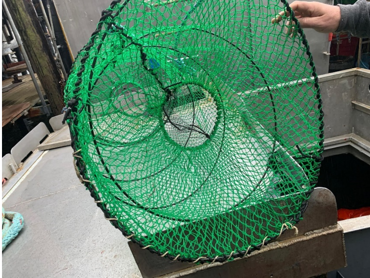
Figure 4-10 Slinky pot with door wrapped closed with cotton twine (white thread on bottom of photo). Proposed in Element 1, currently not allowed by regulation. Source: NMFS OLE, B. Cheeseman.
